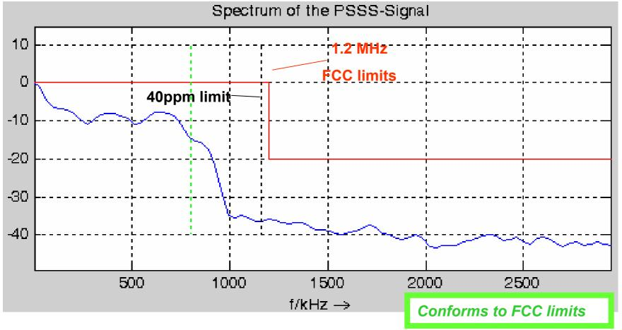
Simulations of the relative PSD in dB for the PSSS signal: With precoding, at 1,600 kchip/s, 250 kbit/s, +/- 40ppm, 100% PA drive, as specified in draft TG4b PHY text
