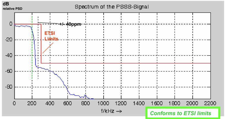
Simulations of the relative PSD in dB for the PSSS 250-400 signal:
