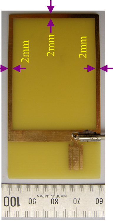
Central portion of ground removed
