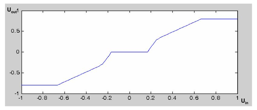
Used transfer function for simulating PSD for non linearity
