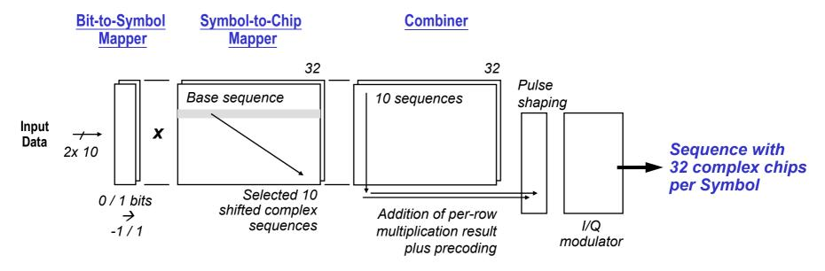
... enables reuse of chip designs with I/Q modulator / demodulator
