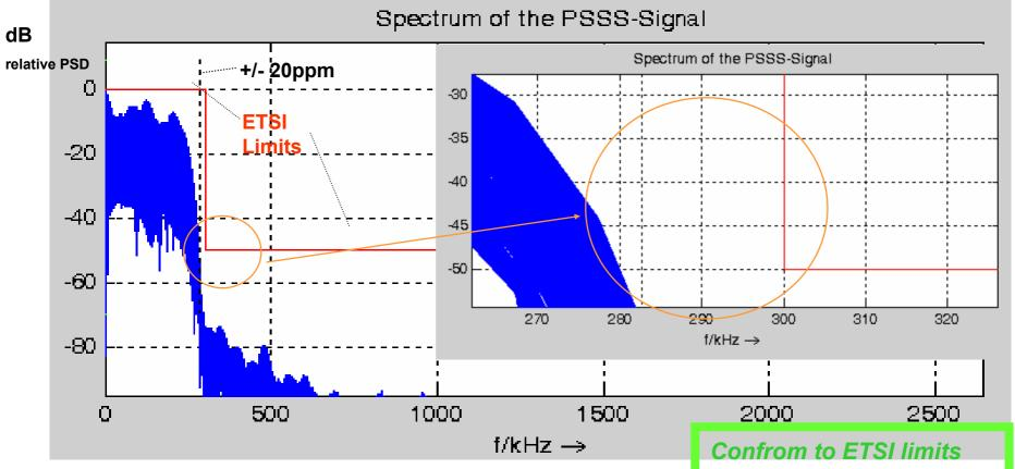
Simulations of the relative PSD in dB for the PSSS signal at 480 kchips/s, 225 kbit/s, +/- 20ppm. Conditions: non linear, no precoding
