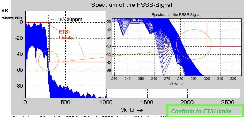
Simulations of the relative PSD in dB for the PSSS signal at 480 kchips/s, 225 kbius, +/- zoppm.
