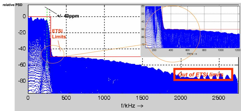
Simulations of the relative PSD in dB for the Cobi at 500 kchip/s, 250 kbit/s, r = 0.2, +/-40 ppm.
