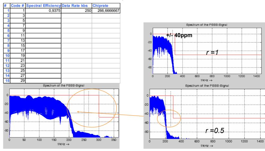
Simulations of the relative PSD in dB for the PSSS signal at 266 kchip/s 250 kbit/s.
