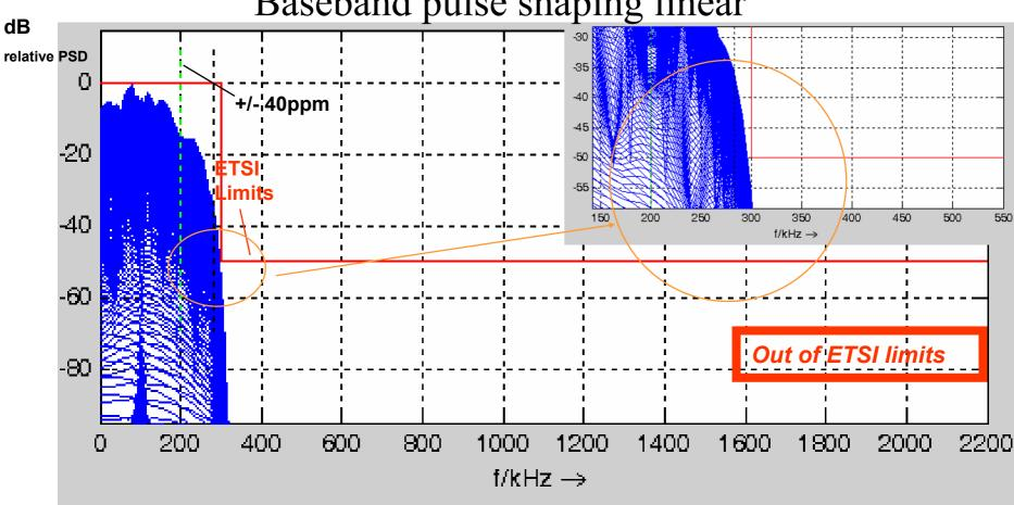
Simulations of the relative PSD in dB for the Cobi at 400 kchip/s, 200 kbit/s, r = 0.5, +/-40 ppm.
