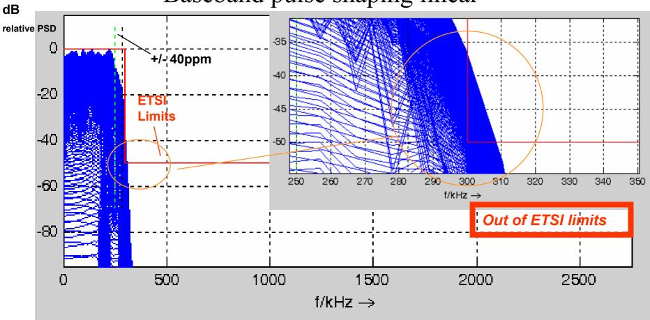
Simulations of the relative PSD in dB for the Cobi at 500 kchip/s, 250 kbit/s, r = 0.2, +/-40 ppm.
