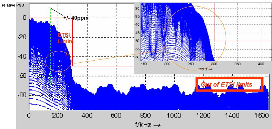
Simulations of the relative PSD in dB for the Cobi at 300 kchip/s, 150 kbit/s, r = 1 + -40 ppm.
