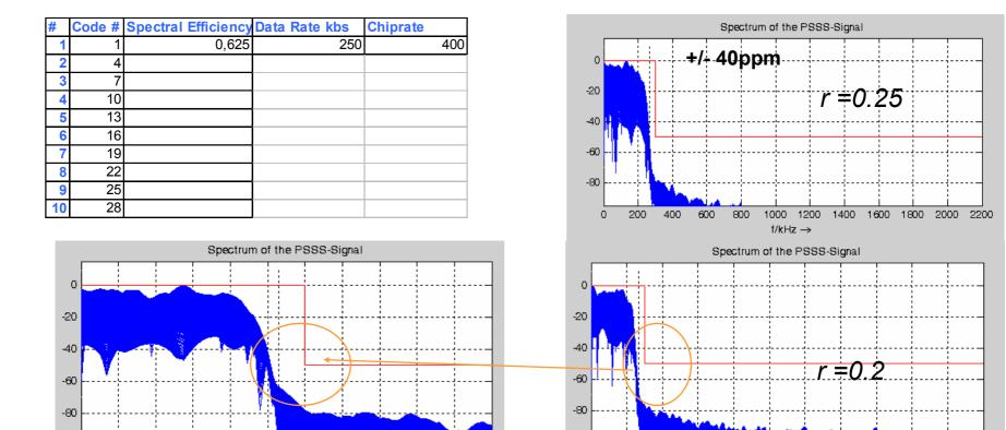
Simulations of the relative PSD in dB for the PSSS signal at 400 kchip/s 250 kbit/s.
