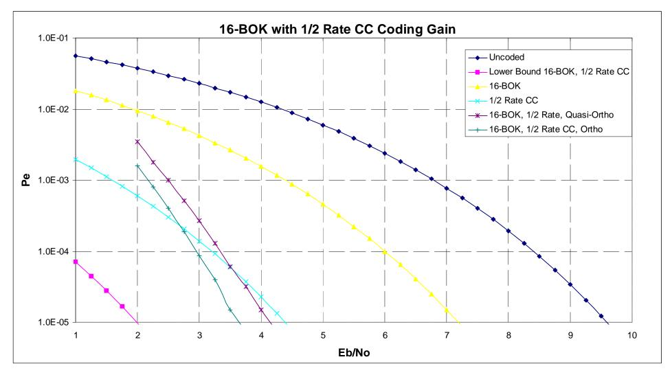
We are falling above the lower bound ... this is due to sub-optimal soft decision mapping of the BOK symbols to bits. This is on-going work and we expect to have this resolved in the near future.
