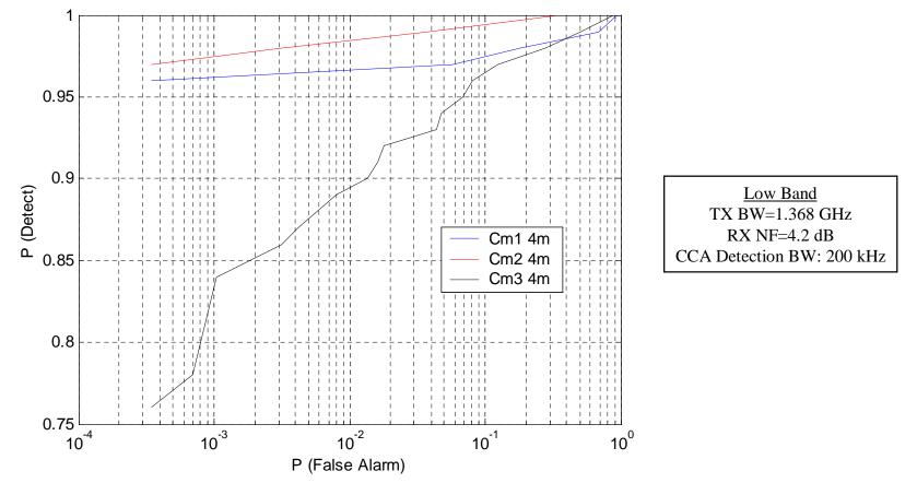
*Our CCA scheme allows monitoring channel activity during preamble acquisition to minimize probability of false alarm acquisition attempts.*
