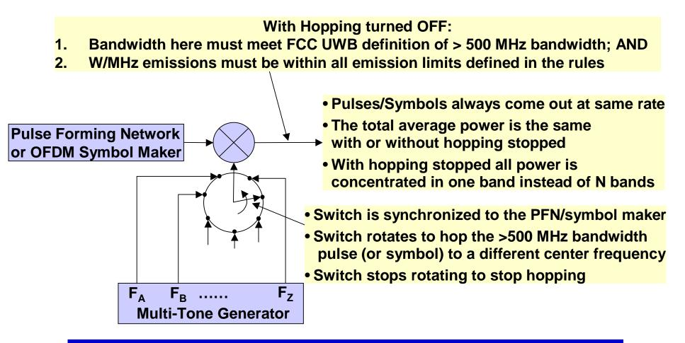
A compliant FH system has only 1/N th the power of a non-hopping system so that it meets the emission limits with hopping turned off
