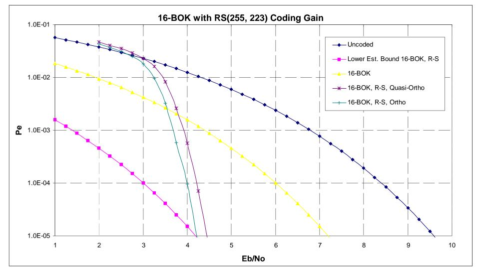
The lower bound estimate was actually done only at 10e-5; so while the lower bound is exact at 10e-5, it is only an estimate above 10e-5. Notice that with orthogonal codes we exactly fall on the lower bound.
