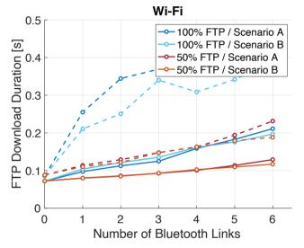
Bluetooth's power backoff increases delays in 100%-load case, but only slightly in 50%-load case
