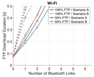
Wi-Fi FTP download operation is completely disturbed by Bluetooth
