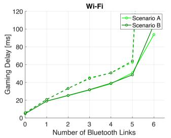
Cloud gaming traffic delay: Significant increase by Bluetooth interference
