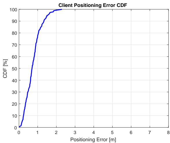
Fig. 12. CToF Client Positioning Error CDF in a Typical Office Environment
