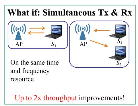
First, hardware must be capable of providing sufficient Self-Interference cancellation!
