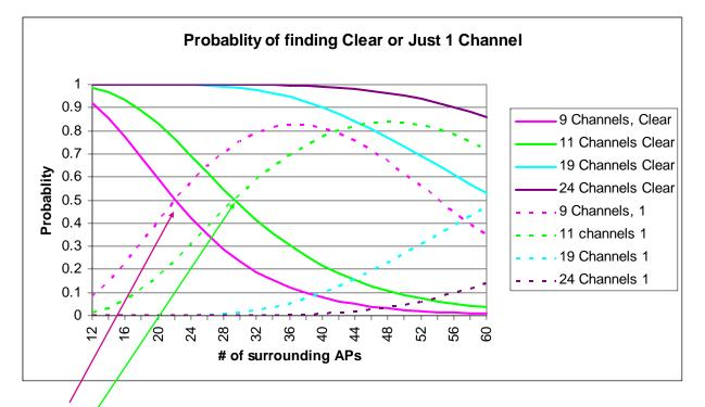
For 9 Channels, with up to 22 surrounding APs, guaranteed to find either clear channel or to share with just 1 For 11 channels up to 29 APs For 19 Channels >60 APs For 24 Channels >60 APs
