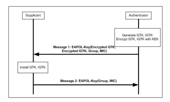
Figure 5-14 — Delivery of subsequent group keys
