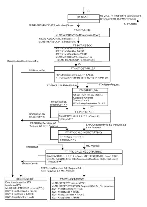
Figure 11A-13—Authenticator R1KH state machine (part 1)
