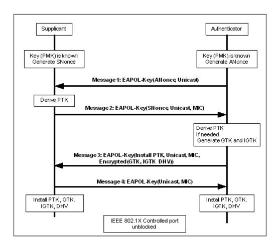
Figure 5-13—Establishing pairwise and group keys
