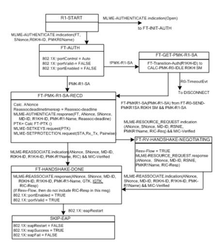
Figure 11A-14—Authenticator R1KH state machine (part 2)
