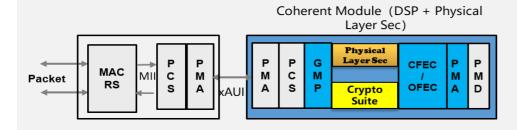
Leveraging the 802.3dj framework, the PAD field within the frame structure may be redefined to carry security encryption parameters (MACSec similar): TCI, AN, PN, SCI, ICV...
