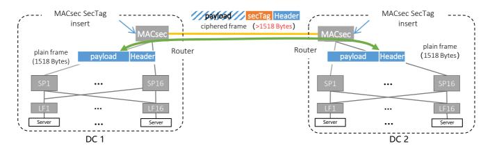
**②** MACsec isn't easy to be deployed at the existed devices without MACsec. MACsec requires parsing upto the MAC layer. Implementing MACsec upgrades necessitates replacement of PHY chips or routing/switching hardware, which entails substantial upgrade costs.
