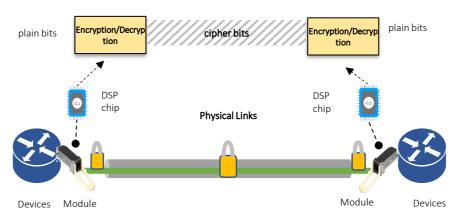
An existing OTN PHY layer security reference: OTN has incorporated physical-layer cryptographic security capabilities (i.e. **FlexOsec**), which uses EOH for security overhead.
