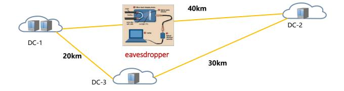
• Encryption of DCI links should be mandatory. The possible methods used to encrypt data of DCI links include MACsec, etc.
