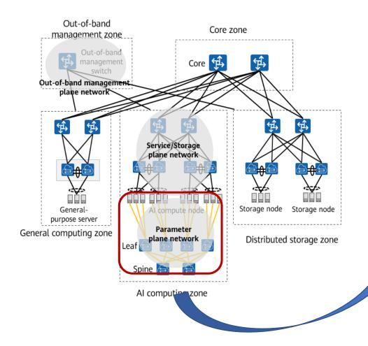
Scale-out network: horizontal expansion to connect more nodes
