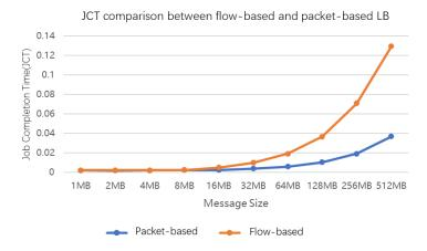
The fine-grained per-packet LB achieve better load balancing effectiveness, but resulting in packets of a flow arriving at receiver out of order. The change from network in-order to out-of-order delivery makes troubles, which mainly in three aspects.
