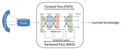
Al large models have to be trained on vast amounts of data. Transformer architecture[9] is the most popular architecture today for Al large model training. It is a set of neural networks consisting of an encoder and a decoder with self-attention capabilities. Analysis in this paper is mainly based on transformer-based architecture.
