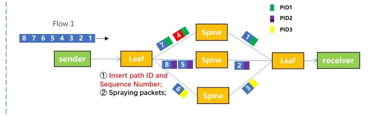
③ Packets of one path arrive the Receiver in order. NIC can quickly detect the loss packet based on the path id and sequence number in a path;
