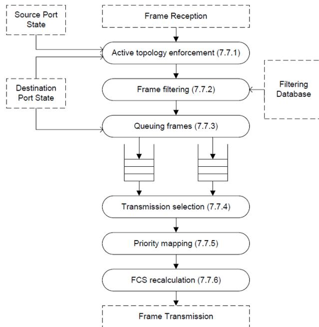
Figure 7-8—Operation of the Forwarding Process
