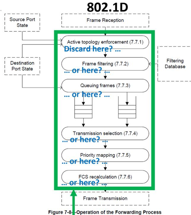
Figure 7-8—Operation of the Forwarding Process
