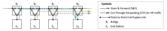
Delay until forwarding to destination port(s). Assumed that the lookup starts after  $l_{Hdr}$  octets and finishes after  $d_{LU}$  µs. Note that the lookup can finish after frame completion during reception.
