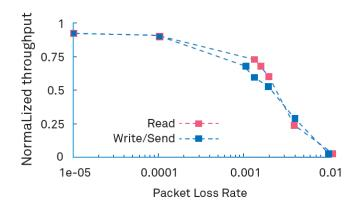
Figure 20 – Impact of packet loss on RDMA throughput
