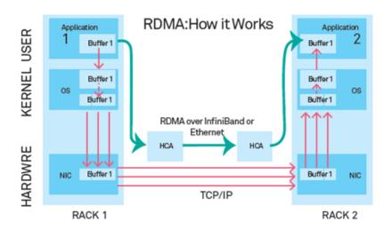
Figure 12 - Working principle of RDMA
