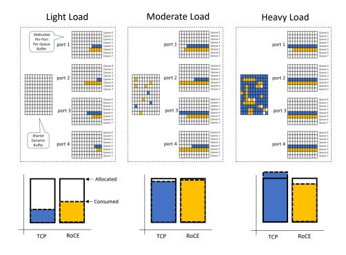
Figure 23 – TCP and RoCE coexistence with smart buffering.
