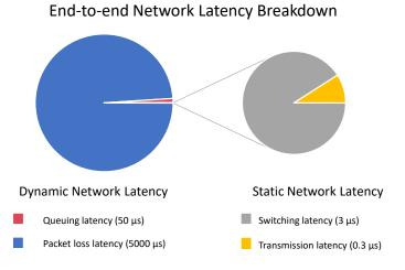
Figure 7 – Network Latency Breakdown
