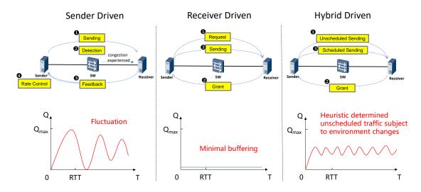
Figure 25 – Transport styles with conceptual network buffering implications
