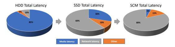
Figure 6 – End-to-end latency breakdown for HDD and SSD
