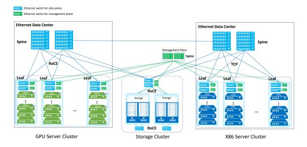
Figure 22 – RoCE application in large-scale data center networks
