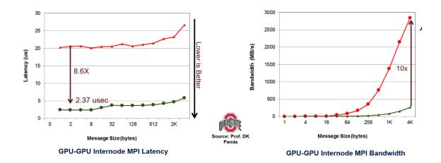
Figure 17: GPU DirectRDMA Performance (From OSU)
