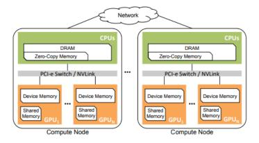
Figure 8 – Distributed AI Computing Architecture
