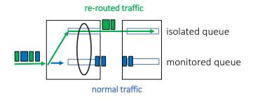
Figure 28 – Queue switch according to CBD reroute flow recognition.
