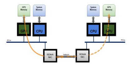
Figure 16: The Data Transfer Using GPU DirectRDMA
