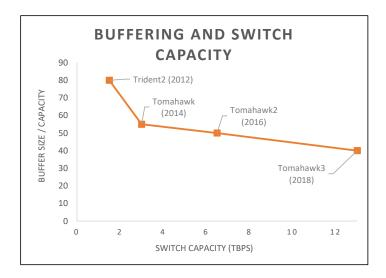
Figure 18 – Switch Chip Buffer Trends
