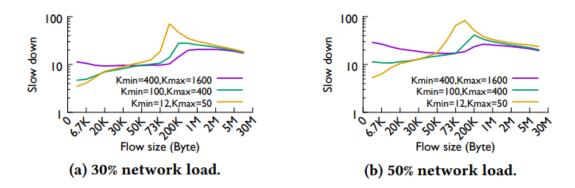
Figure 19 – FCT slowdown distribution with different ECN thresholds, using WebSearch
