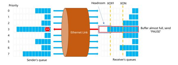
Figure 24 – Priority-based Flow Control (PFC)
