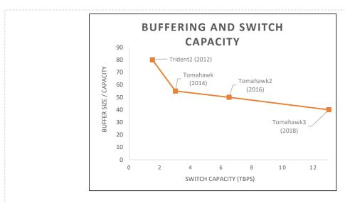
Figure 18 – Switch Chip Buffer Trends
