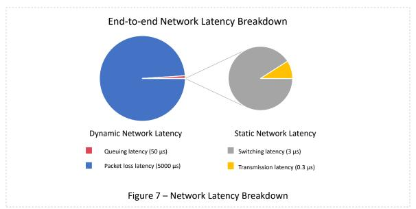
The major component of dynamic latency is the delay from packet retransmission when packets are dropped within the network. Packet loss latency is an order magnitude greater than queuing delay and has proven to have a severe impact on applications. Figure 7 shows a typical network latency distribution.
