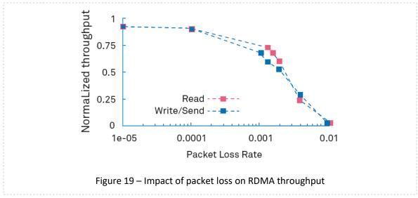
center network. Figure 19 from [20] shows how RoCE service throughput decreases rapidly with an increase in the packet loss rate. Loosing as little as one in one thousand packets decreases RoCE service performance by roughly 30%.
