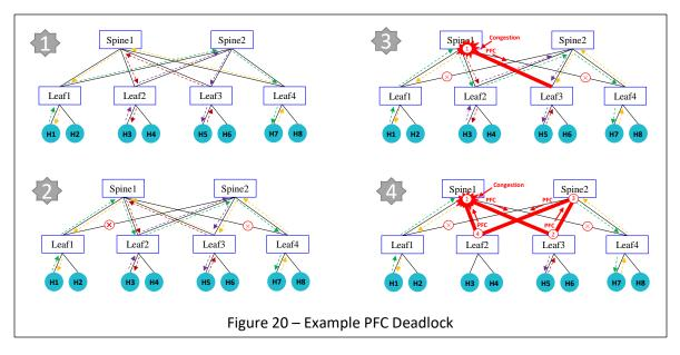
lowest latency. While there are no loops in the logical topology, these paths naturally contain loops in the physical topology. A PFC deadlock in the network can completely halt network traffic.
