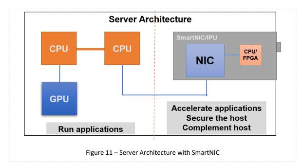
SmartNICs in the data center increase the overall utilization and load on the network. They can exacerbate the effects of congestion by fully and rapidly saturating a network link. At the same
