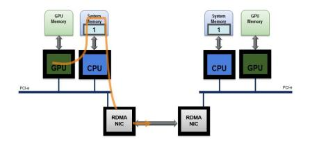
Picture 15: The Data Transfer Based On GPU Direct
