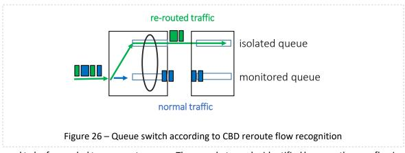
need to be forwarded to a separate queue. These packets can be identified because they are flowing from a port oriented as an uplink to another port oriented as an uplink. Figure 26 illustrates the process of queue remapping within the switch. In the example, the remapping of the green flow to an isolated queue will lead the elimination of PFC deadlock. The different flows can safely pass through different queues at the point of a potential CBD.
