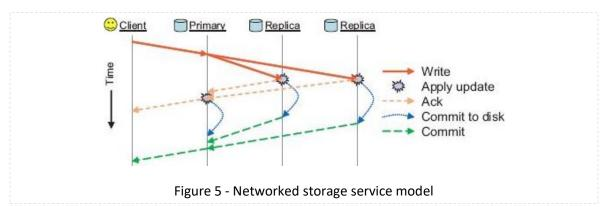
The example highlights the importance of the network enabling both high throughput and low latency simultaneously. The bulk data being written to the primary storage server is transmitted multiple times to the replicas. The small sized acknowledgments and commit messages must be
