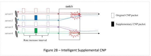
The ODCC tested the enhanced congestion control mechanism and the effect is beneficial [25]. According to the test result, the bandwidth QoS performance is improved by more than 30% (TCP:RoCE = 9:1 scenario).
