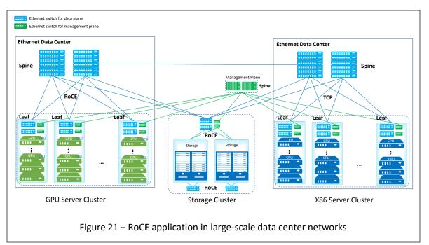
In the large-scale data center network scenario TCP and RoCE traffic can traverse common parts of the network in several different ways:
