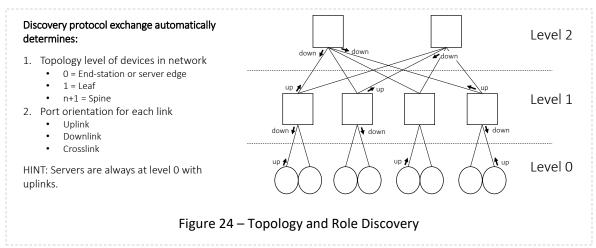
The protocol starts out by recognizing known conditions. Servers and storage endpoints are always at level 0 and their port orientation is always an uplink. Switches are initialized without any knowledge of their level or port orientation, but as the information is propagated by a discovery protocol, the algorithm converges upon an accurate view. Figure 24 shows the resulting topology and role discovery in a simple Clos network.
