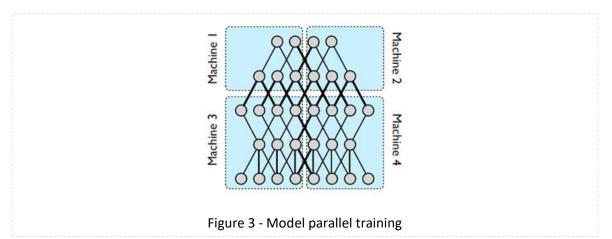
estimate for all the data parameters. With model parallel computing, there is an initial distribution of the common data set to a distributed number of nodes, followed by a collection of individual parameters from each of the participating nodes. Figure 3 shows how parameters of the overall model may be distributed across computing nodes in a model parallel mode of operation.
