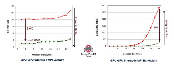
Figure 17: The Performance Of GPU DirectRDMA (From OSU)
