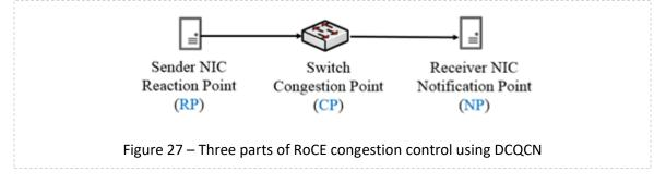
Congestion is determined by looking at the egress queue length and evaluating it against configurable thresholds ( $K_{min}$  and  $K_{max}$ ). When the queue length is less than  $K_{min}$ , traffic is not marked. When the queue length is greater than  $K_{max}$ , all packets passing through the queue are marked. When the queue length is between  $K_{min}$  and  $K_{max}$ , the marking probability increases according to the extent of the queue length, as specified by DCQCN.
