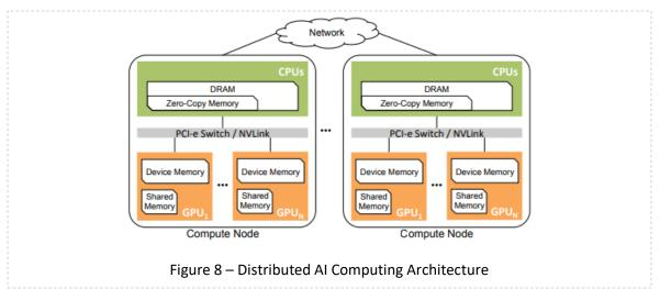
Facebook recently tested the distributed machine learning platform Caffe2, in which the latest multi-GPU servers are used for parallel acceleration. In the test, computing tasks on eight servers resulted in underutilized resources on the 100 Gbit/s InfiniBand network. The presence of the network and network contention reduced the performance of the solution to less than linear scale [12]. Consequently, network performance greatly restricts horizontal extension of the AI system.
