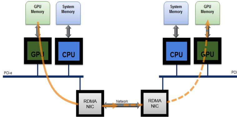
**Figure 16: The Data Transfer Based On GPU DirectRDMA**
