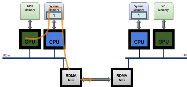
**Picture 15: The Data Transfer Based On GPU Direct**
