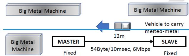
**Figure 13** Layout in factory for which measurement of RSSI is recorded
