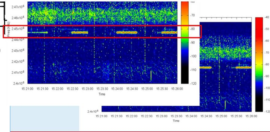
**Figure 47** Wireless signals with coexistence of different wireless technologies. The x- and horizontal axes show frequency (Hz) and time, and color shows signal strength in a bar on the right hand side.
