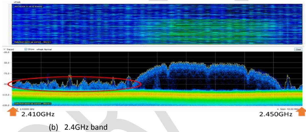
**Figure 5 Measured noise spectral density within (a) 1.9 GHz band and (b) 2.4 GHz band**
