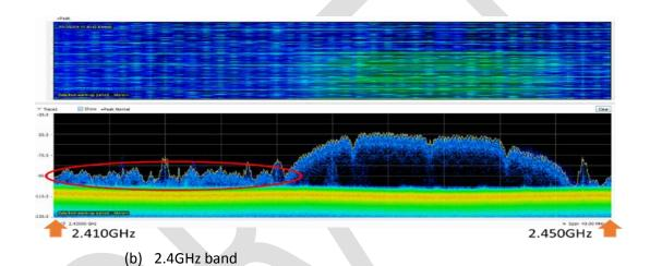
Figure 5 Measured noise spectral density within (a) 1.9 GHz band and (b) 2.4 GHz band
