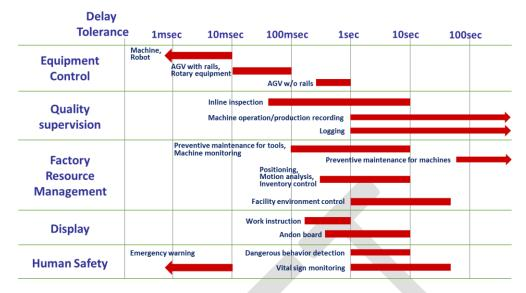
Figure 11 Permissible latencies of representative wireless applications
