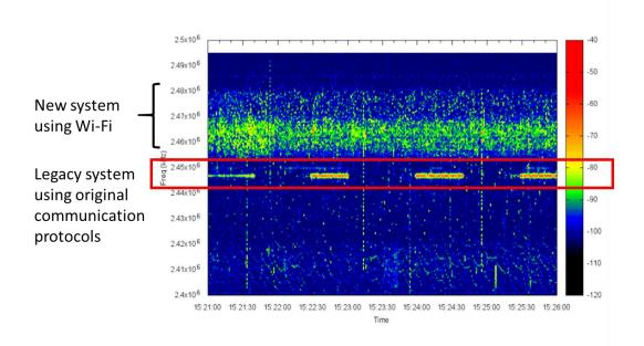
Figure 7 Coexistence of different wireless technologies
