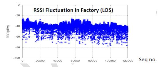
Figure 4 RSSI Fluctuation in Factory (LOS)
