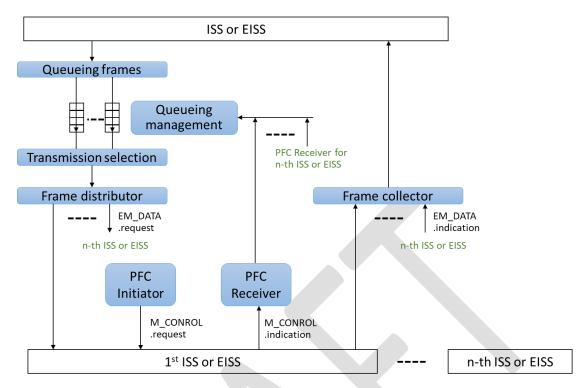
Figure 18 PFC aware system queue functions with Link Aggregation (Rewritten Figure 36-4 in Std. 802.1Q-2014)
