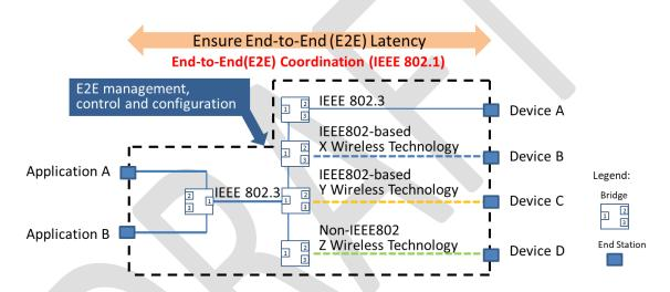
Figure 2 Example of Network Topology in Factory Environment
