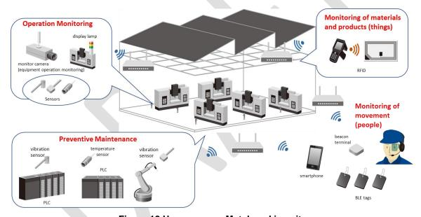
Figure 12 Usage scene: Metal working site
