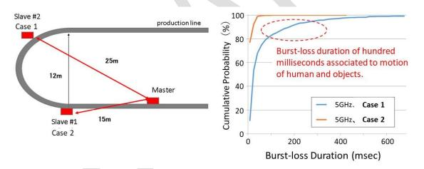
Figure 17 Burst-loss measurement in a large machine assembly site [2]
