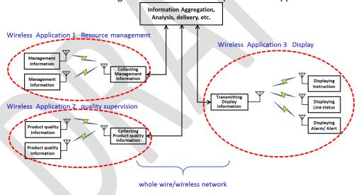
Figure 9 Scope of wireless applications in factory
