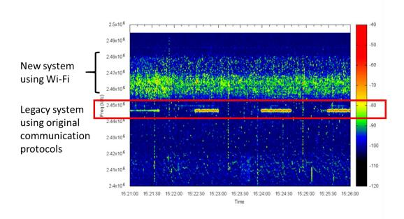
Figure 7 Coexistence of different wireless technologies
