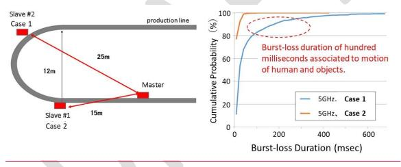
Figure 17 Burst-loss measurement in a large machine assembly site [2]
