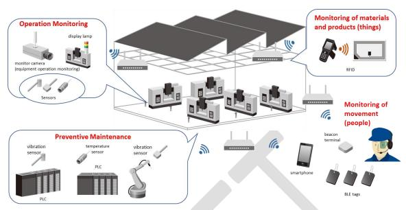
Figure 12 Usage scene: Metal working site
