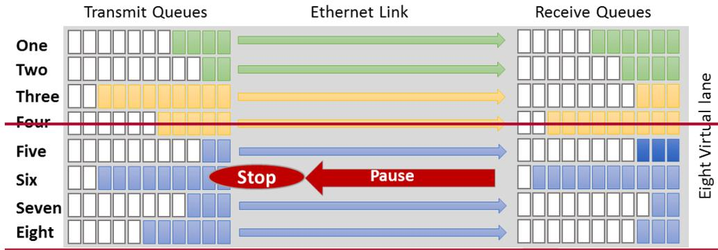
**Figure 16 Example of operation of the PFC function**
