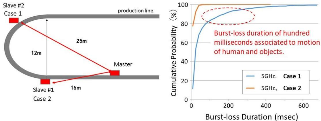
**Figure 17 Burst-loss measurement in a large machine assembly site [2]**
