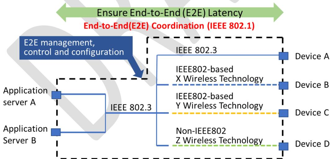
Figure 2 Example of Network Topology in Factory Environment
