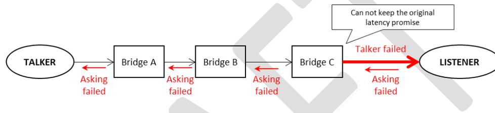
**Figure 16 Radio fluctuation causes reservation failed**
