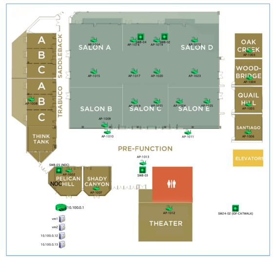
Figure 1. Twenty-four access points were deployed throughout the meeting space.
