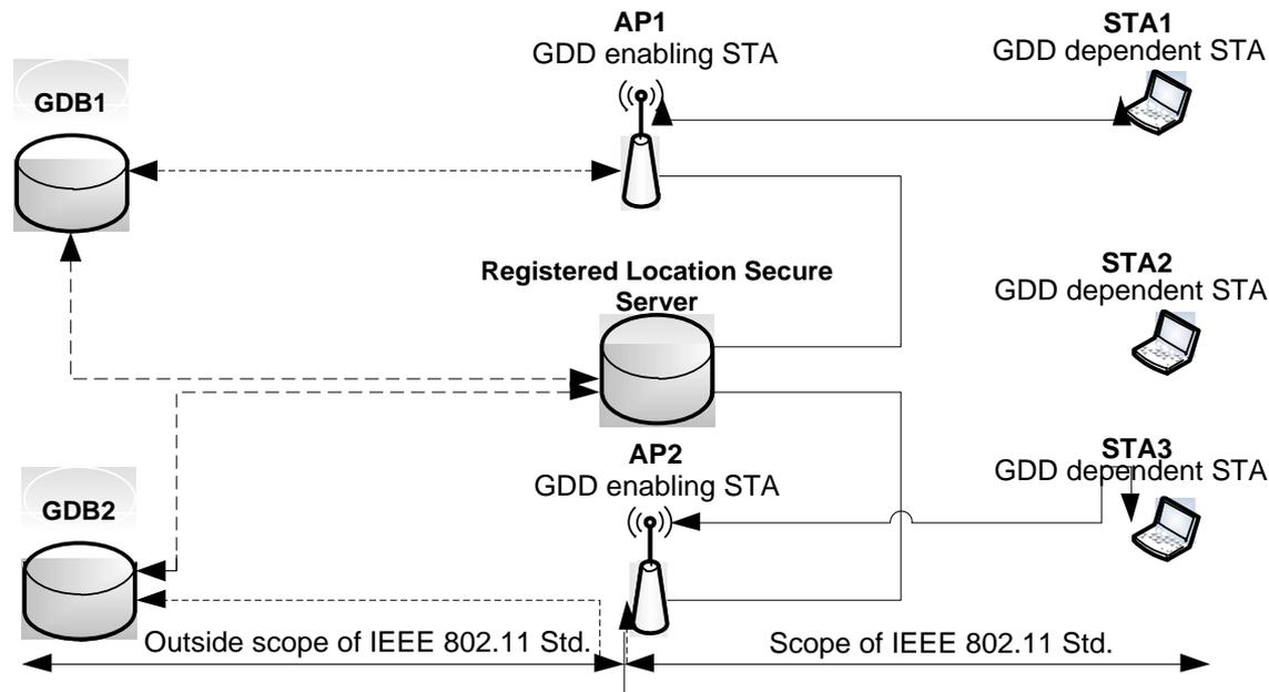
The RLSS provides the database function for multiple networks. It can access a regulatory database, or using centrally mounted antennas, provide available channel information based on sensing of the spectrum.
