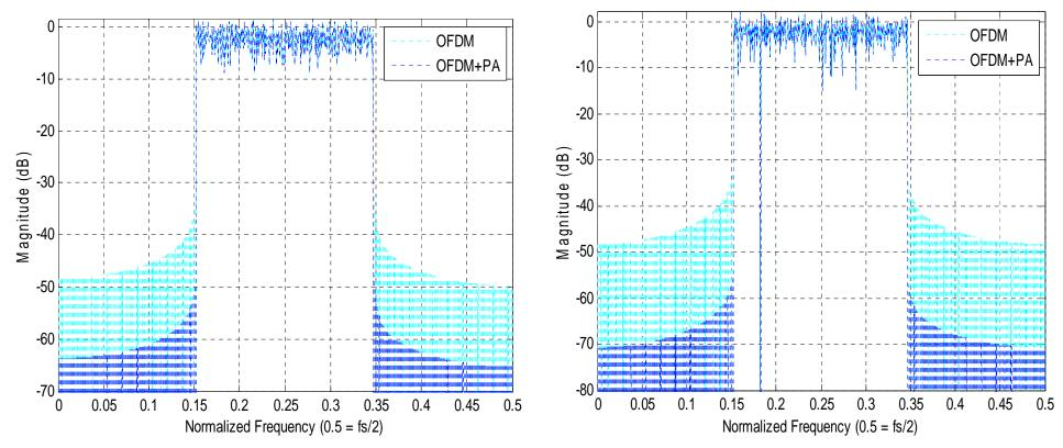
➡ For both urban and suburban area, the power spectrum of incumbent receiver in adjacent channels are further degraded with pathloss considered.
