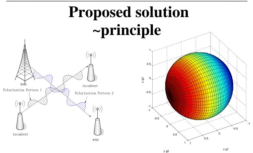
→ The power is totally received (red) when polarization states matched and little is received (blue) when mismatched.
