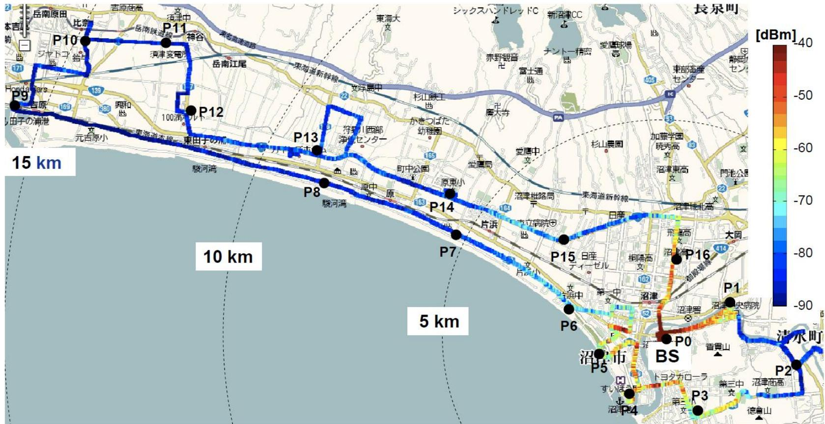
•Site measurement of received power vs. distance with base station antenna height: 45m
